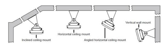
Mounting brackets are included with your purchase for easy installation in a variety of positions. Depending on the area and the available space, you may want to mount the heater on either the wall or the ceiling.
